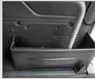
STORAGE COMPARTMENT Side storage compartment made of thermoformed ABS plastic
