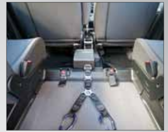
F-WINCH Allows drawing the wheelchair onto the access ramp, in a comfortable and safe way
